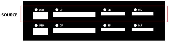
Use only one of the USB, CF, SD or MS slots on the top row as the source and one of the slots at the 2nd row below as target for duplication. Do not plug in 2 or more USB and memory cards as source or target at the same time.
