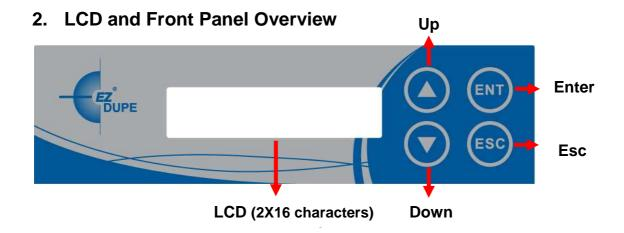
**▲ Button:** *Up, Backward:* To navigate backward in the menu. **▼ Button:** *Down, Forward:* To navigate forward in the menu.
